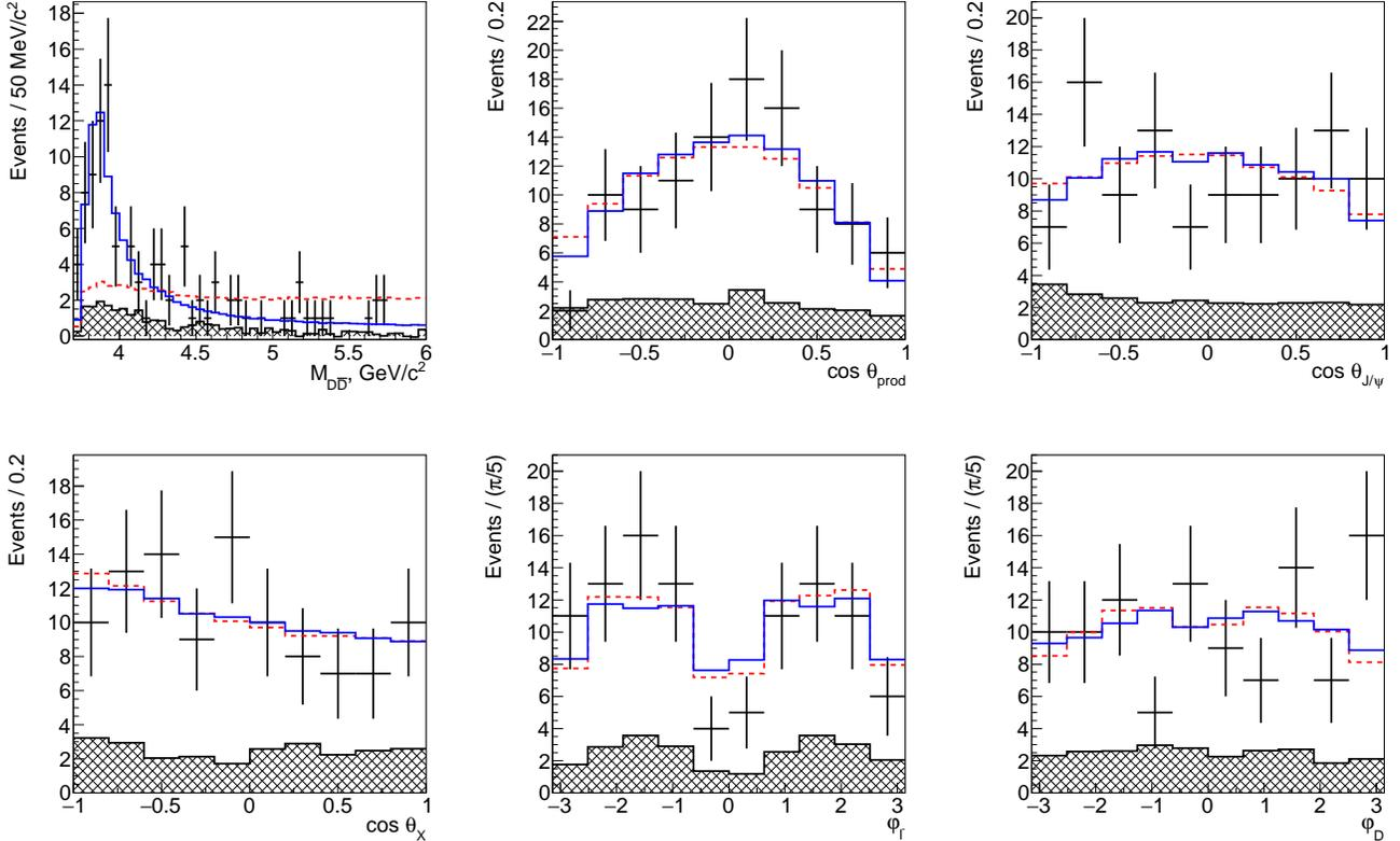
FIG. 6. Projections of the signal fit results in the default model onto  $M_{D\bar{D}}$  and angular variables. The points with error bars are the data, the hatched histograms are the background, the blue solid line is the fit with a new  $X^*$  resonance ( $J^{PC} = 0^{++}$ ) and the red dashed line is the fit with nonresonant amplitude only.
