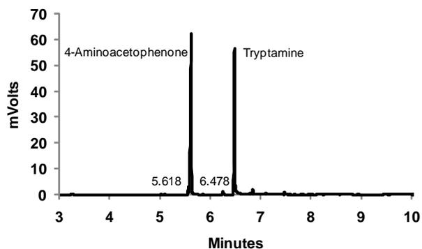
**Figure 2.** Representative GC/FID chromatogram of an extracted, spiked sponge sample.
