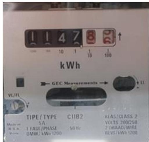
**Figure 6: Electricity meter with kWh output** (Zietsman, 2015)
