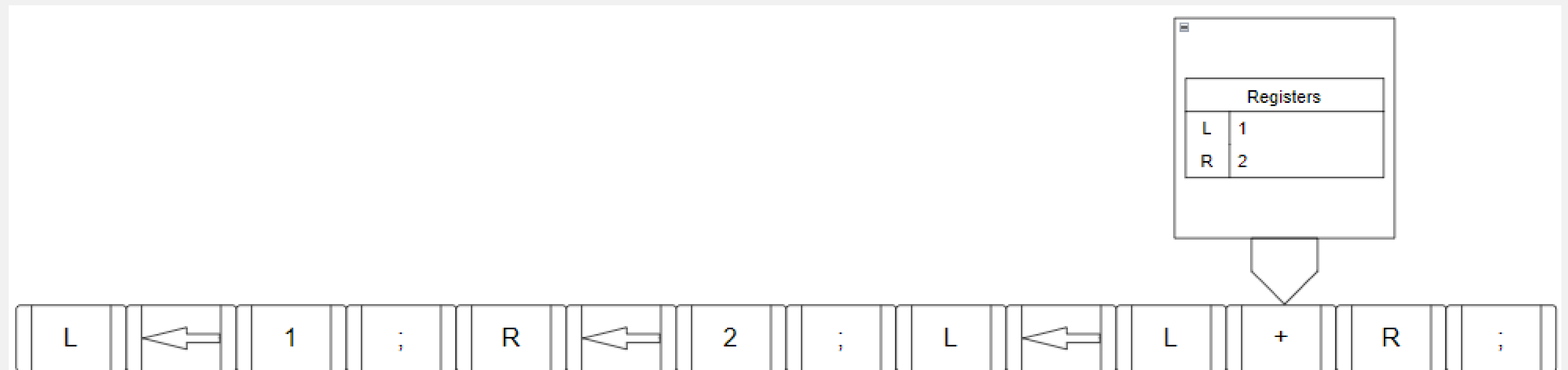
Fig.1 An abstract LRT machine computing the expression 1+2
