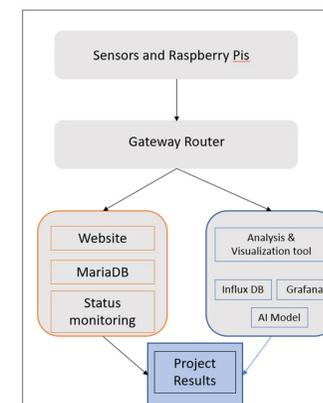
Figure 4 - Data Transfer Process
