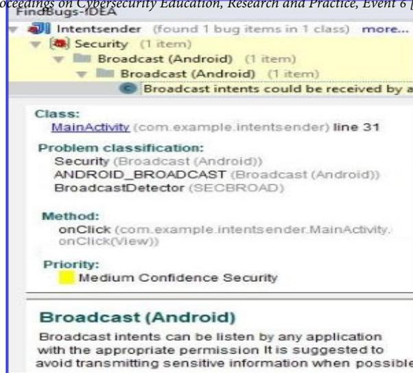
**Figure 3: Broadcast intent detected by FindSecurityBugs**
