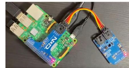
Fig: Prototype consist of Raspberry Pi4 connected to a BMP180 pressure sensor that transfers the data using a 12C Shield digitizer.
