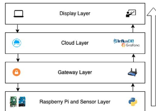
Fig: Architectural framework for collecting data from IoT devices
