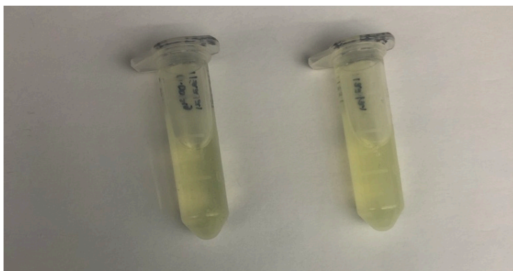
Figure 16. Reaction tubes after 1,10-phenanthroline was added to PaIVY reacted with [\text{Re}(\text{CO})_3(\text{H}_2\text{O})_3]\text{X}^+ ( 1 ) indicating the formation of the warhead ( 3 ) due to the yellow color.
