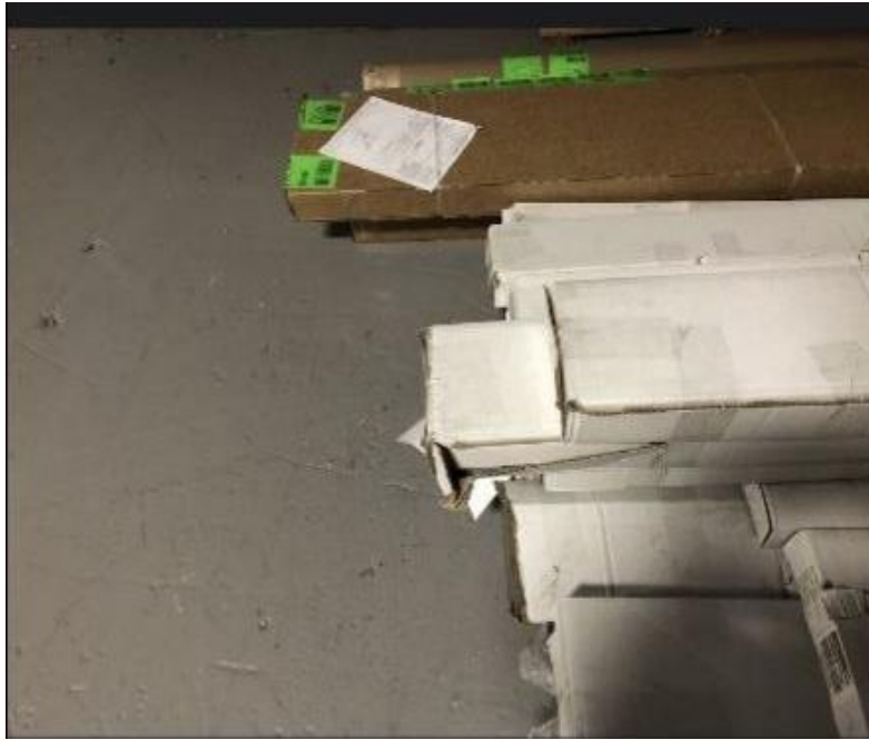
Figure 1 Depicts damaged vinyl flooring packages
