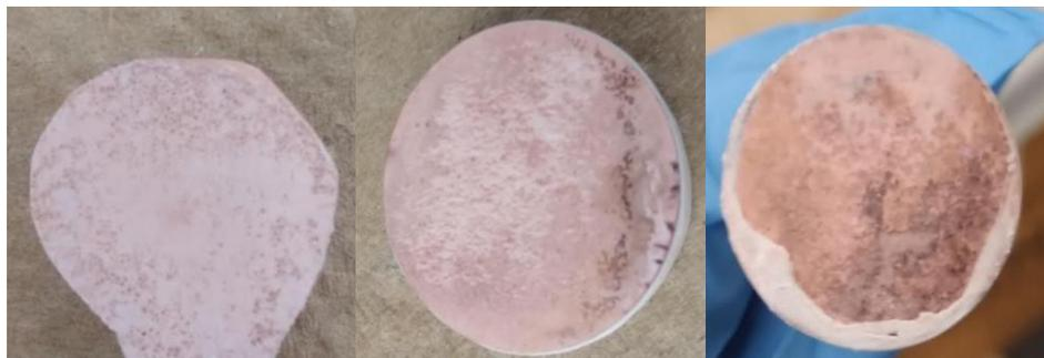
**Fig. 3.11** Image of HA/Cu sample with 0.80 mM SDS with pH adjustment of 5.80 (A), 1.80 mM no pH adjustment  $\sim$ 4.3 (B), and 0.80 mM no pH adjustment  $\sim$ 4.3 (C).
