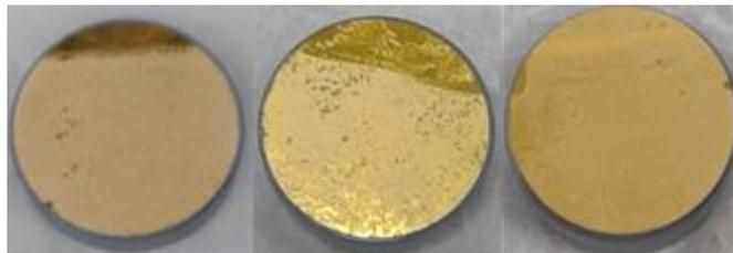
**Fig. 4.10** Image of HA films on gold-plated flat mirrors show improvement in surface coverage. From left to right: samples W, AA, and AG. Synthesis conditions are listed below in Table 4.5.
