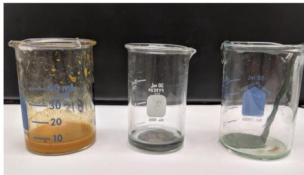
**Fig. 4.7** Image, from left to right of iron, stainless steel, and nickel in UAFW. These experiments were heated to 65°C and all metals reacted in solution with ammonia.
