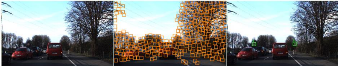
Figure 2: (Left) The input image. (Middle) The extracted ROIs. (Right) The output image with detected traffic signs.
