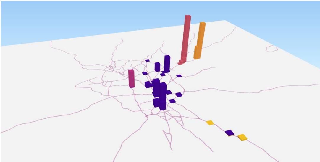
Figure 27: Plot of Clusters indicating sum of congestion events throughout the sampling period. The plotted data is an indicator of temporal severity of congestion clusters.
