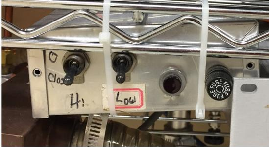
5. Start mechanical pump with ON/OFF switch.
