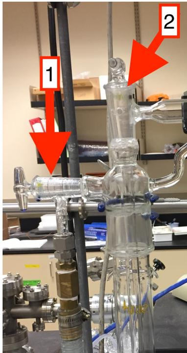
14. Start a very low flow rate of carrier gas (typically UHP N<sub>2</sub>) from gas cylinder.
