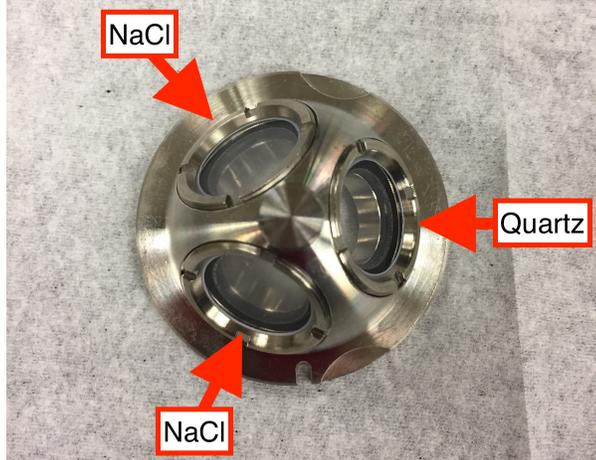
a. Remove windows from dome using “tool”, shown below.
