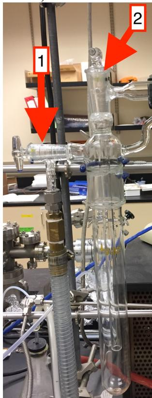
2. Open mixture bulb and allow pressure to stabilize throughout the manifold.
