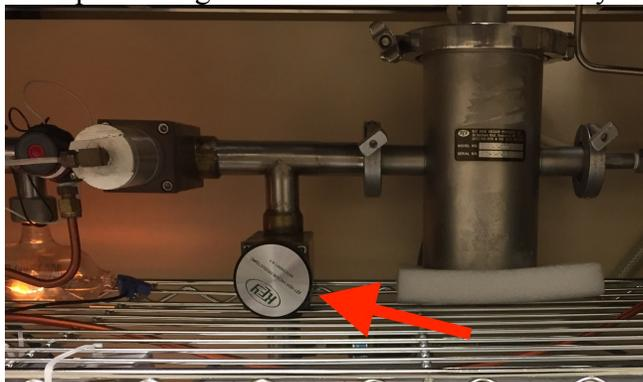
7. Slowly open the bellows valve from vacuum manifold to DRIFTS cell. Pressure in cell, shown on the PC, should be allowed to reach 3-5 torr and maintained there throughout the duration of the experiment by continually opening the bellows valve until it is fully open, and then by using the needle valve on the vacuum manifold.
