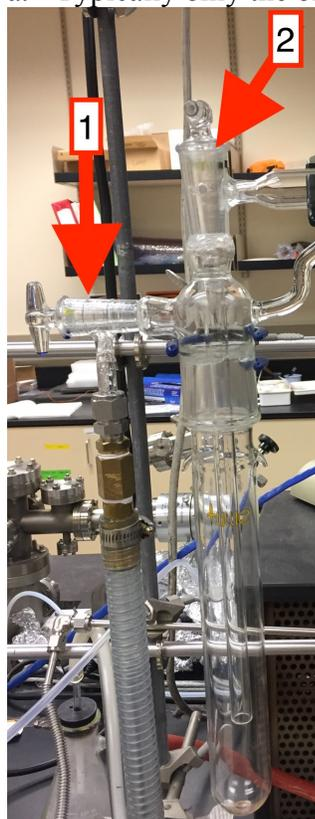
6. Once evacuated leak check the manifold by closing the valve on top of the manifold (2) and watching for any rise in the pressure.
