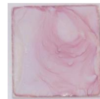
FIGURE 2.3 The “coffee ring effect” during AuNP drop casting
