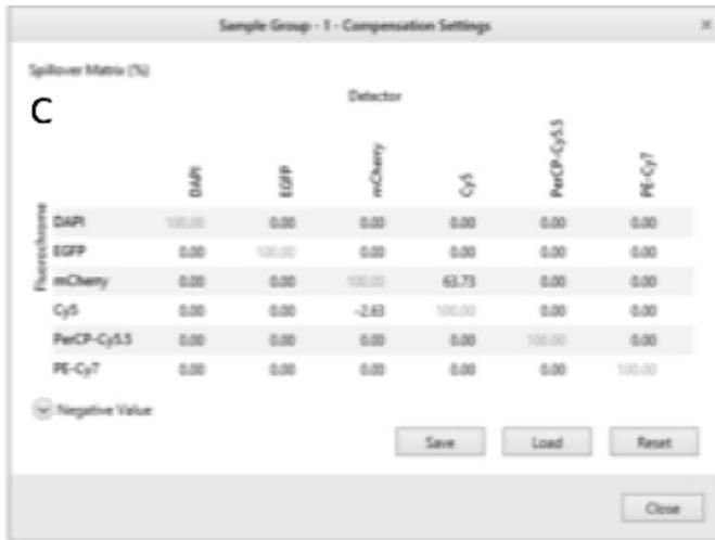
**FIGURE 21: Applying Manual Color Compensation Calculation Matrix**
