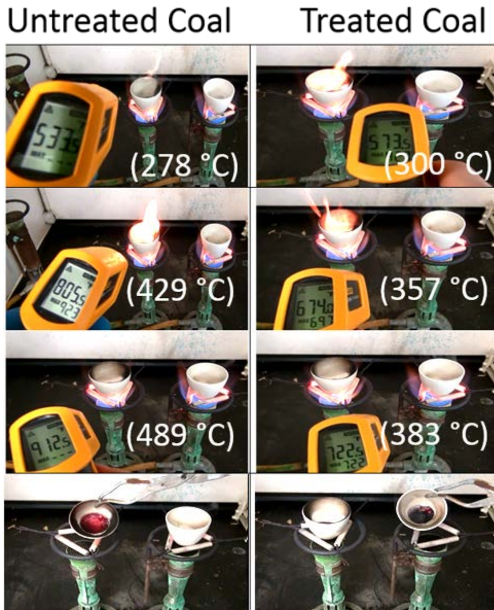
Figure 5. Flammability Test of Untreated and Treated Coal
