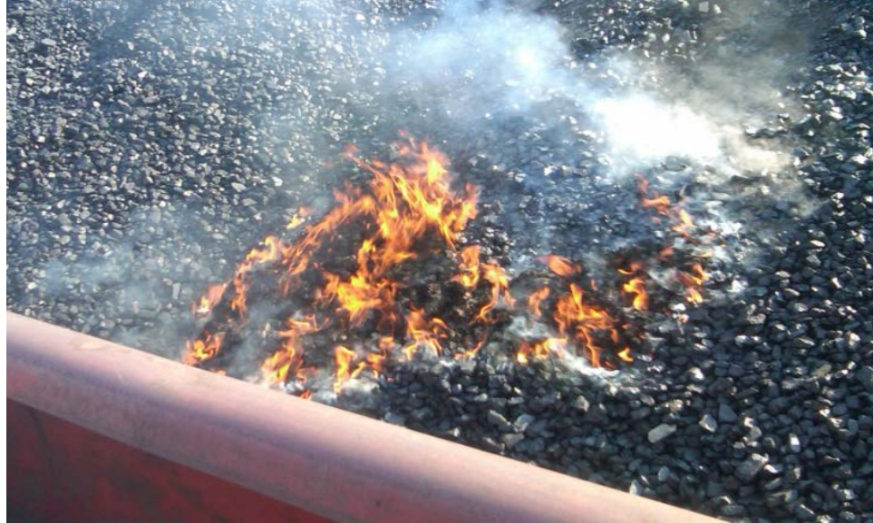
Figure 2. Sub-bituminous Coal that has Spontaneously Combusted
