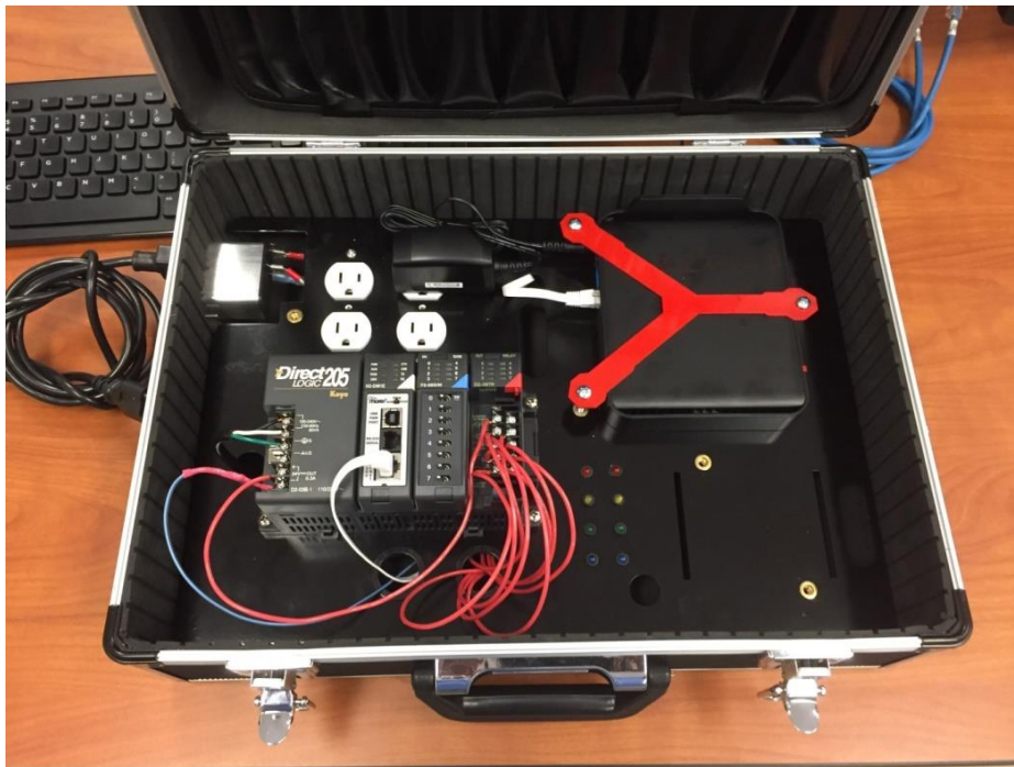
Figure 1. The Industrial Control Systems Toolkit
